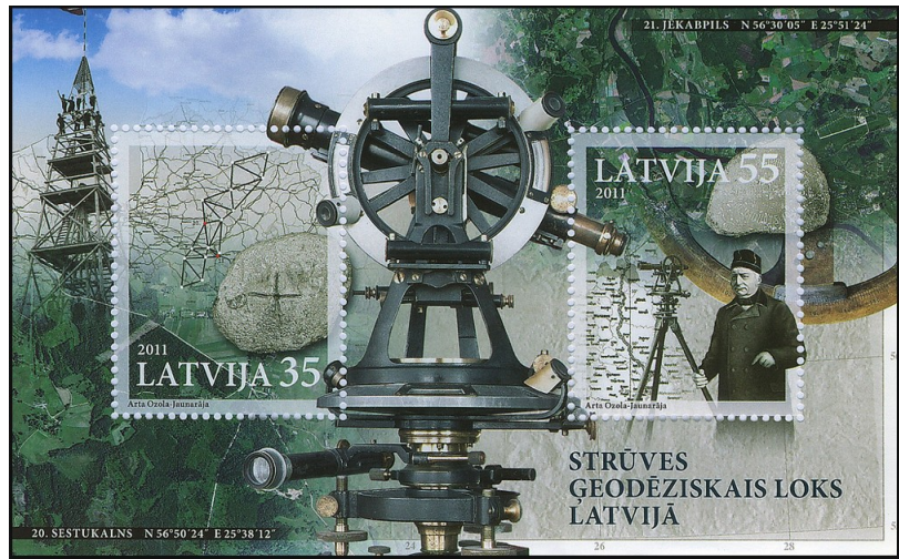
Fig 14 Struve Arc with chain of triangles, wooden trigonometric tower on a mountaintop, and theodolite for measuring the angles in the triangles (Latvia 2011).
