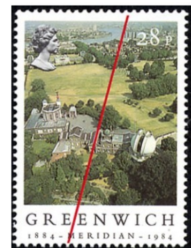
Fig.19 The WGS84 Zero Meridian runs 336 feet east (right) of the red line (old Prime Meridian of 1884). GB Sc. 1060.
